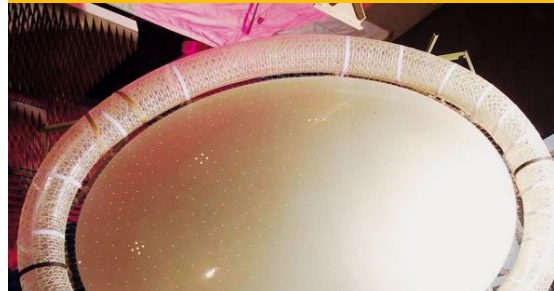
1 Inflatable 4x6-meter communications antenna concept
