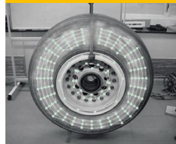
1 Experimental setup and scan grid on the A320 wheel (courtesy Groupe SOPREMA, Vélizy, France)
