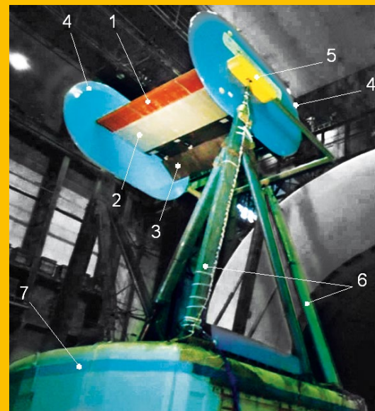
2 The prototype wing section in the working portion of the wind tunnel (1 - adaptive slat, 2 - caisson, 3 - flap, 4 - fin, 5 - fairing, 6 - aerodynamic support scales, 7 - aero-dynamic stall scales)
