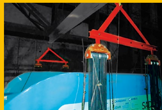
3 Elastic support system for prototype frequency experiments
