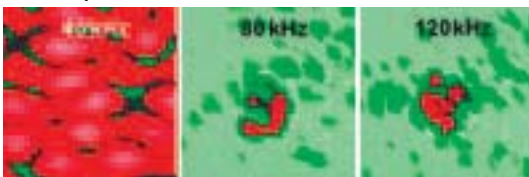
Non-destructive testing of delamination in a composite material
