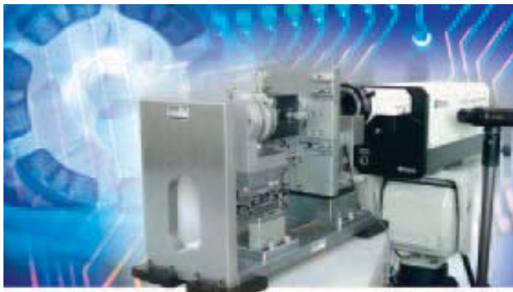
Noise investigation in hard disk spindle motors using scanning vibrometry
