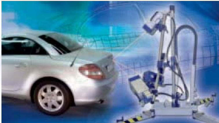
3-D scanning measurement of structural dynamics of a car body
